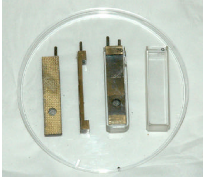
Figure 4.2.4.1: purpose built tissue holders used to hold sheets of retina in the light path of the spectrometer, within a standard 10 x 10 mm cuvette.
