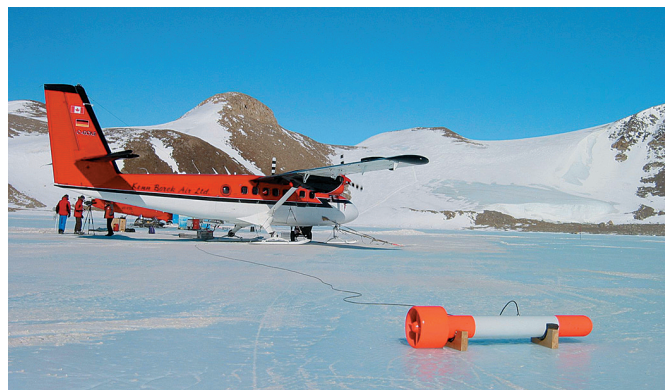
Fig. 7: Installation and ground testing of the aeromagnetic equipment in the survey Twin Otter on the sea-ice in Tethys Bay – the innermost part of Gerlache Inlet – close to the Italian Mario Zucchelli Station.
