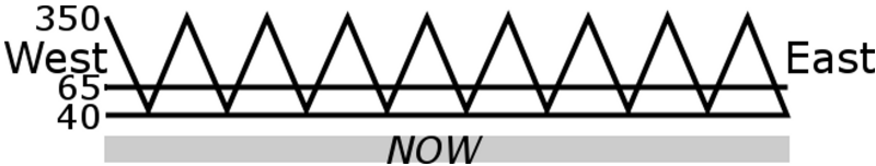
Figure 3.6: NOW flight strategy of the cross-profiles. Lateral view.
