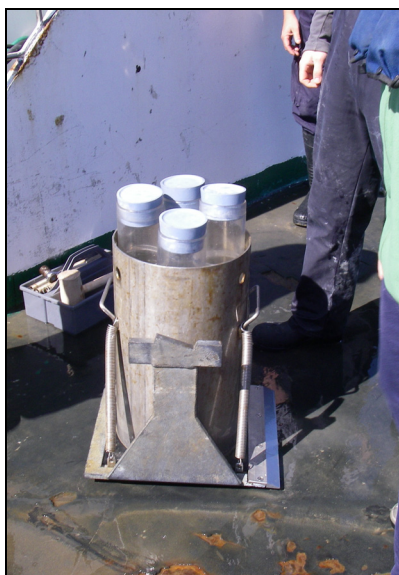
Figure 3: Retrieval of the cores. Sub-sampling of the BC with the MUC cores
