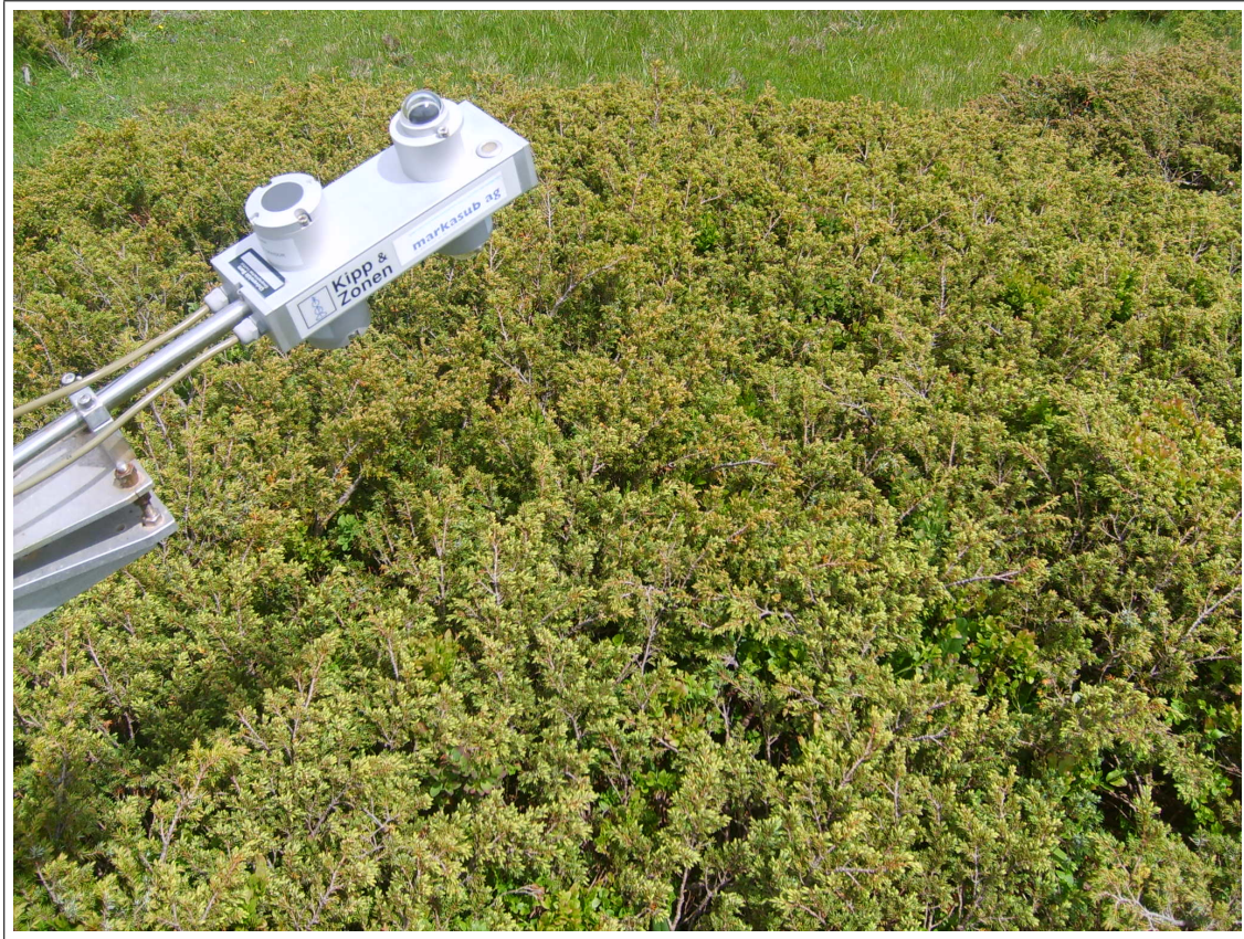
Figure 4: The instrument (Kipp & Zonen CNR1 Net Radiometer) at its measurement position over the Juniper shrub area. Albedo was measured with the two sensors having a transparent quartz glass dome (one sensor looking upwards, the other downwards). The two sensors with a flat dark filter glass are the pyrgeometers for long-wave radiation measurements.
