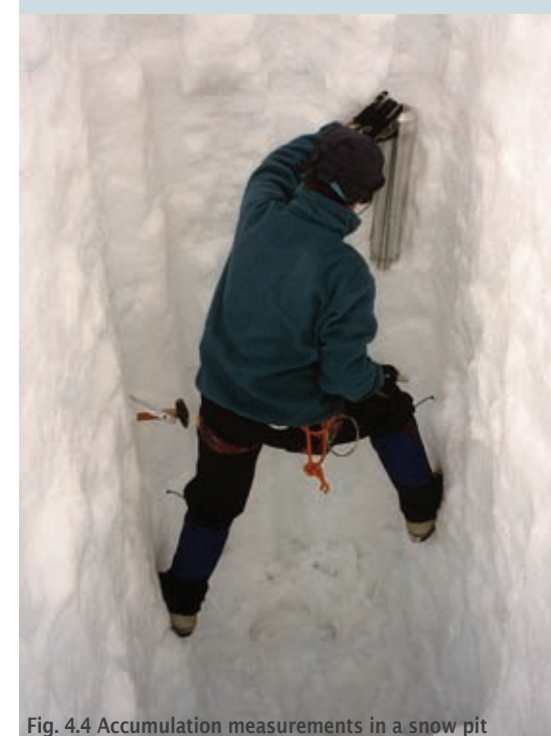
Fig. 4.4 Accumulation measurements in a snow pit
