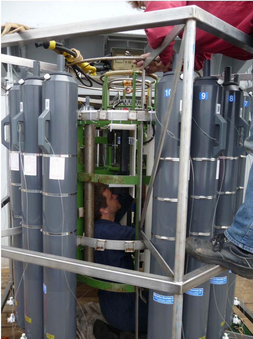
Figure 3: Underway repair of the CTD by Lorendz Boom (inside the frame) and Martin Laan, searching for the problem, which in the end proved to be a leaking cable.
