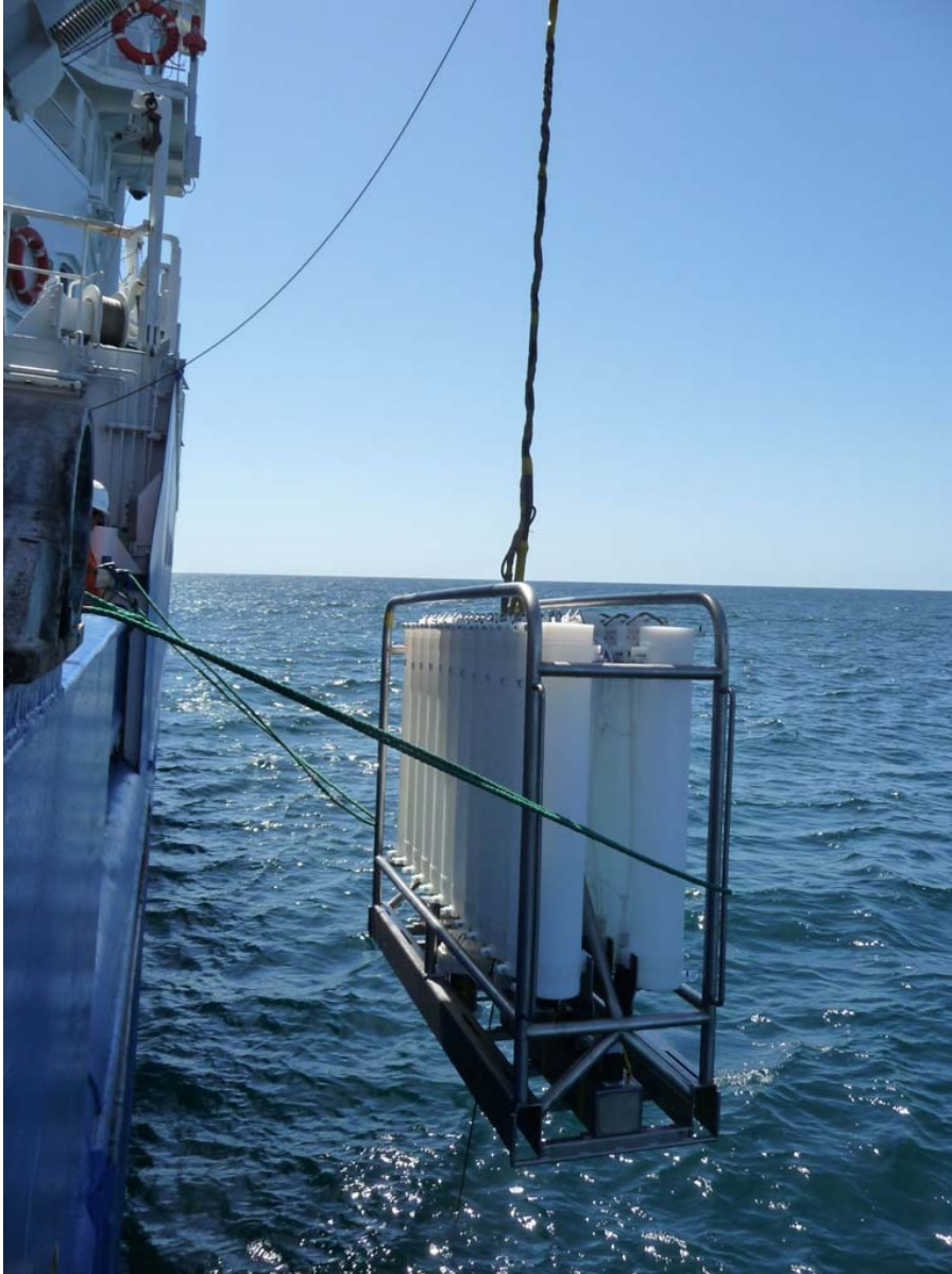
Figure 2: the Ultra Clean CTD hanging next to the starboard side of Pelagia.
