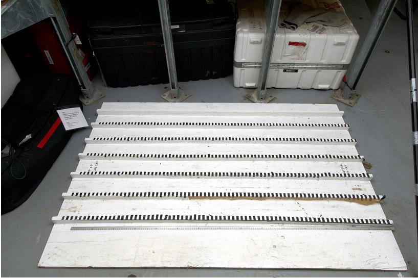
Figure 8. Manufactured photography table for placing core sections.
