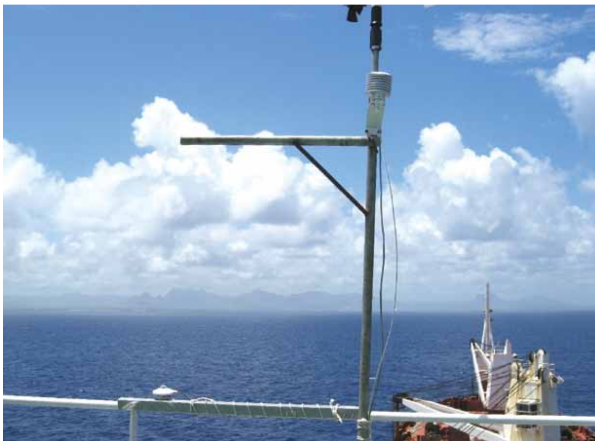
Fig.5.3-6. Weather parameters were recorded along the ship track by using an Automatic Weather Station installed on onboard MV Emerald Sea during the 26th Indian Scientific Expedition to Antarctica (2006–2007) for IPY project no. 70.
