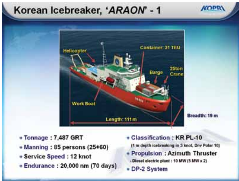
Fig.5.3-16. Major technical and research parameters of Araon .
