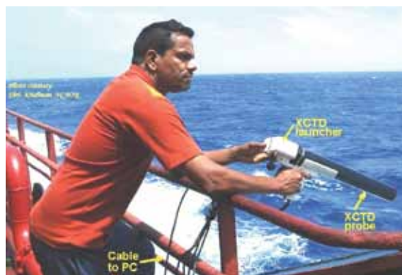
Fig.5.3-5. The data collection campaign for IPY project no. 70 launched in austral summer 2007. Project PI, Alvarinho J. Luis launches an XCTD probe in the Southern Ocean.
