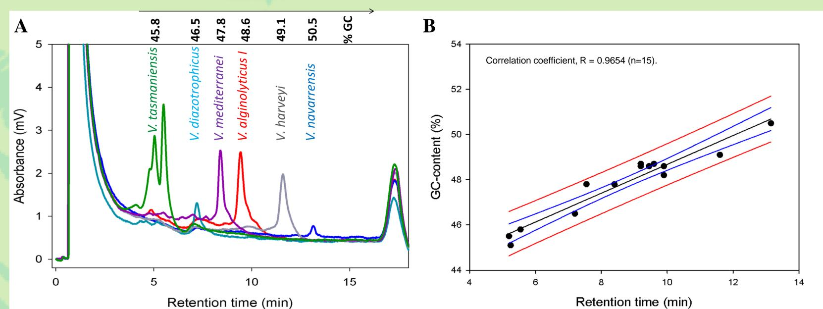
**Figure 4:** DHPLC analysis of individual PCR-products of 6 Vibrio species amplified with primer-set 5 (with GC-clamp). Acetonitrile gradient: 45 % Buffer B for 0 min (loading), 54 % B for 2 min to 60 % B for 14 min at 63.5 °C; flow rate 0.9 ml/min; injection volume 10 μl (A). Retention time observed in the DHPLC analysis was correlated with GC-content of the *rpoB*-sequences (B).
