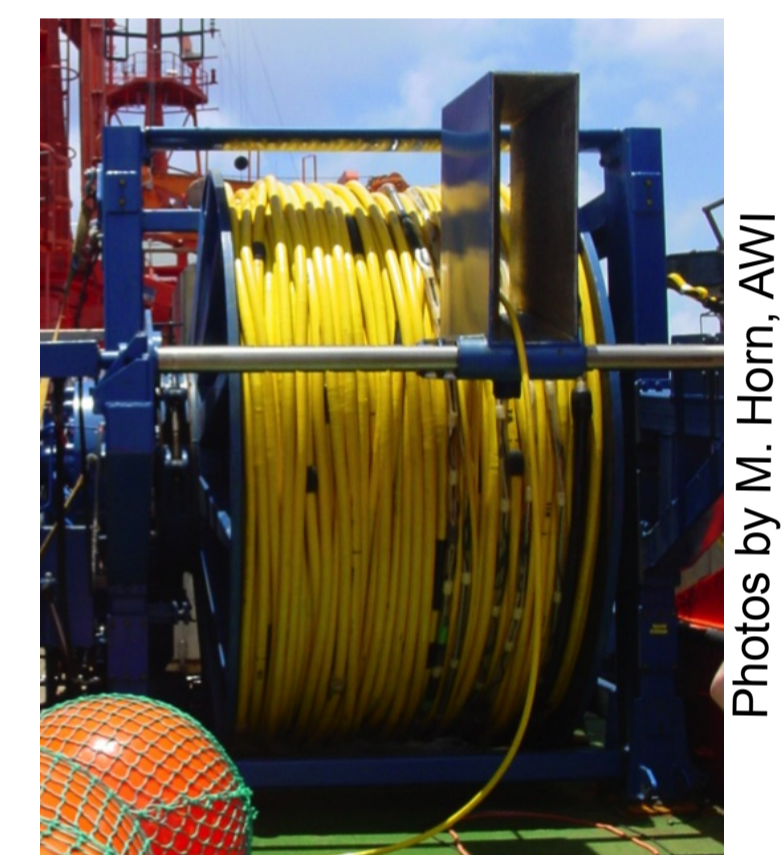
Fig. 5 Receiver: Streamer with hydrophones
