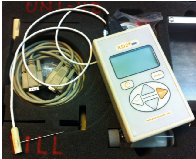
Fig. 8.2: KD2 – Pro thermal properties analyzer. Picture shows handheld device, powered by 4 AA batteries, and the 6 cm single needle sensor. The sensor is directly inserted into the sediment.
