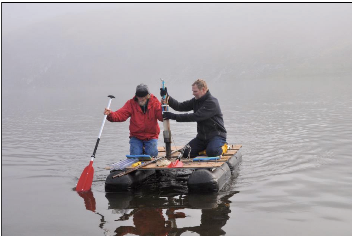
Fig. 12.6: Small platform used for the coring of fresh-water lakes, here with a gravity core retrieved on Jason Lake A
