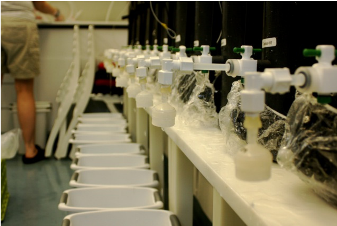
Figure 2. Swinnex 25 mm filter holders showing 3/8" OD tubing, 90° compression-NPT adapter, and NPT-Luer lock adapter. Note 11 L waste baskets for filtrate volume measurements.
