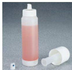
Figure 7. Nalgene Aerosol Spray Bottle has no metal parts, and can be acid cleaned
