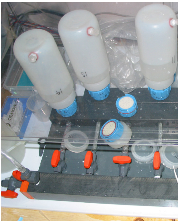
Figure 3. An example of a 1 L offline filtration method as used routinely on CLIVAR A16N, A16S, VERTIGO, and GEOTRACES IC expeditions. Pre-cleaned 1L LDPE bottles are modified with closing air vents at bottom. Sample is quickly transferred from the GO-Flo into the 1 L LDPE bottle which is then capped conventionally. Once returned to a Laminar Flow bench environment, the top is substituted for a tapered adaptor which has a mated 47 mm MFS filter holder with preloaded 0.45 \mu\text{m} Supor filter. The upstream orifice of the filter holder has been drilled out to twice standard diameter to minimize air-lock effects. Once samples are filtered under 25 to 40 mm Hg vacuum, they are transferred directly to sample bottles for further processing. Primary sample bottles and filter holders are reused after TM-clean DI water rinsing. More information available from J. Bishop ( jkbishop@berkeley.edu ) or Todd Wood ( tjwood@lbl.gov ).
