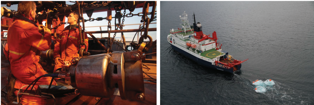
Figure 2.2: (Left) G-Gun used during ARK XXV/3. (Right) A cluster of six G-Guns and two additional G-Guns are towed by Polarstern during the seismic refraction survey of ARK XXV/3. Fotos from M. Koch, 2010.
