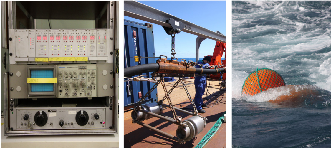
Fig. 3.2: Impression of the airgun operations at sea. From left to right: the triggerbox unit, providing the electric pulse to fire the G-guns; G-gun cluster, hanging in the deployment frame on the aft deck; flotation buoys to maintain a fixed depth of the airguns in the water.
