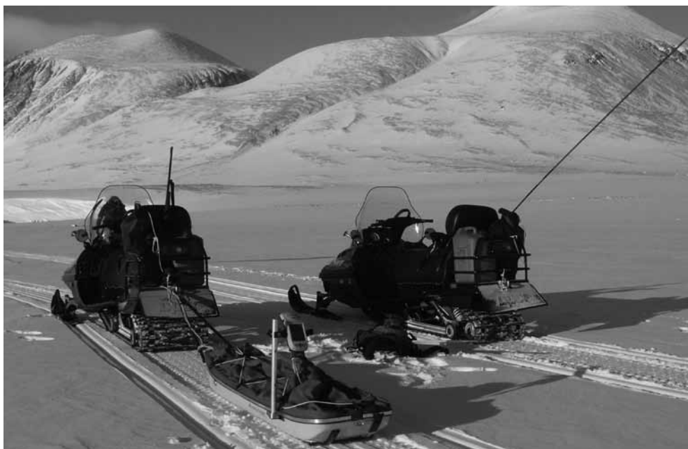
Figure 2.9 The GPR was set up with the 500 MHz shielded antenna and batteries in a sledge hooked to a snow mobile. The Ramac X3M screen was attached on the steer of the snow mobile to enable the driver to control the instrument. Manual snow depth measurements were made at regular intervals.
