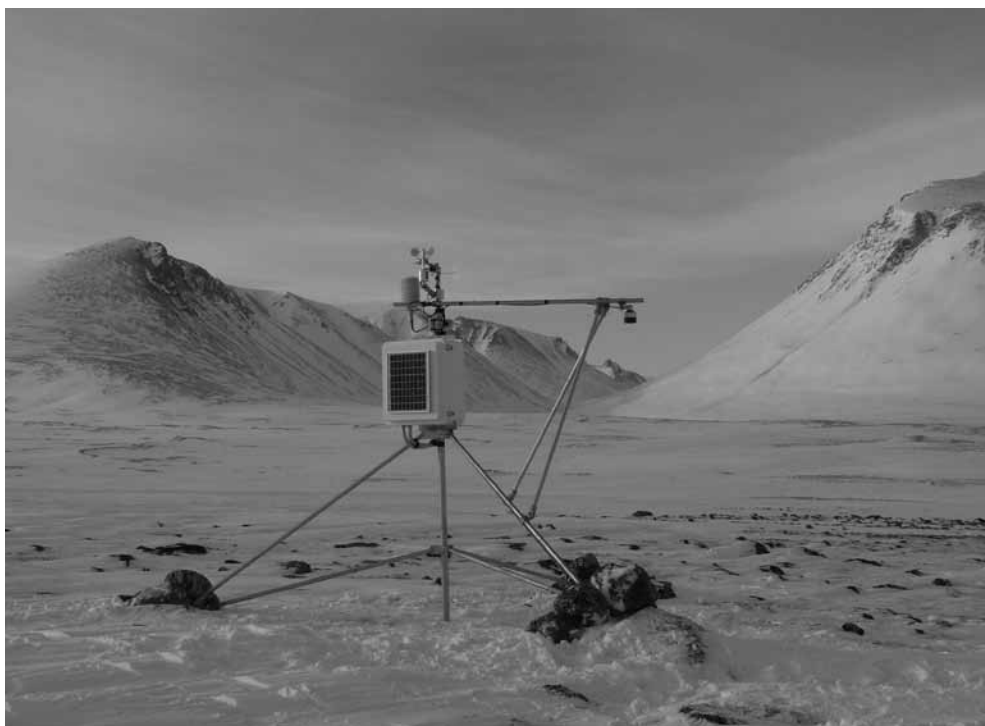
Figure 2.4 The new automatic weather station in Store Sødal (M7), 21 March 2008. Photo: Charlotte Sigsgaard.
