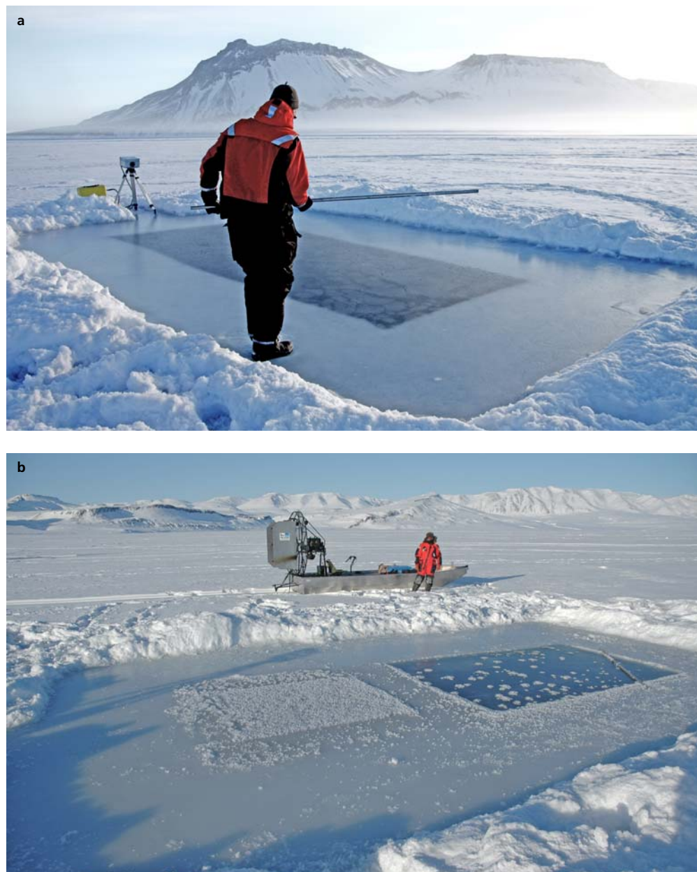
Figure 6.32 Opening cut for a) the in situ frost flower growing experiment and b) the frost flowers formed on new ice overnight. Photo: Jakob Sievers (top) and Søren Rysgaard (bottom).
