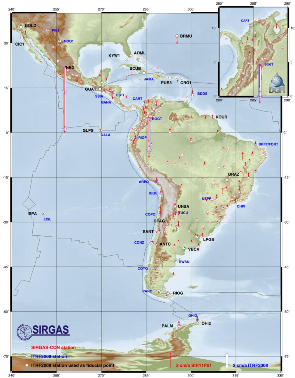
Fig. 14. Vertical velocities of the SIR11P01 multi-year solution. Velocities of ITRF2008 stations are included for comparison.
