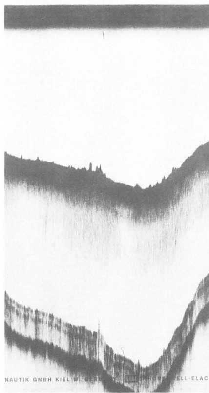
Fig. 5 (a, b + c) Indication of wrecks, rock peaks and fish in echo and double echo
