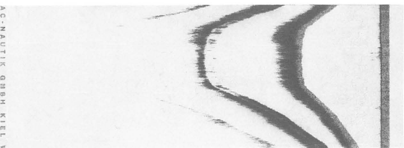
Fig. 4 Decrease in number of multiple echoes with increasing depth
