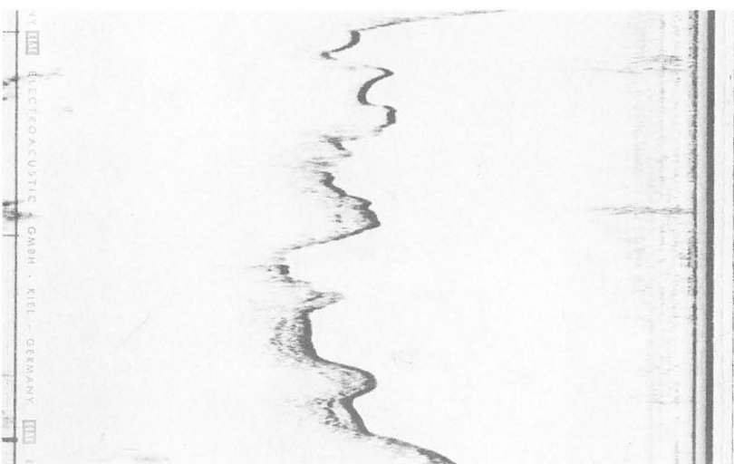
Fig. 8b Indication of formation of ground at low gain
