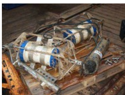
Fig. 11b: The retrieved instruments are overgrown by organisms. (They appreciate oceanographic moorings just
