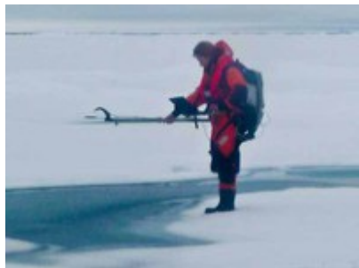
Fig. 5: Larysa Istomina measures light reflection by a spectral radiometer. (© AWI Sea Ice Physics)
