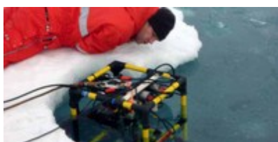
Fig. 5: In situ analyses of under ice primary production and respiration - will the fine microsensors last for the deployment? (© M. Fernandez)
