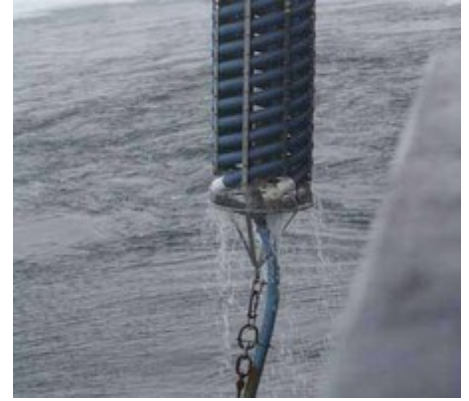
Fig. 7: Retrieval of a mooring component. This is called the "chick" - a device enabling water column profiling without using batteries, what a great idea! (© B. Rabe)
