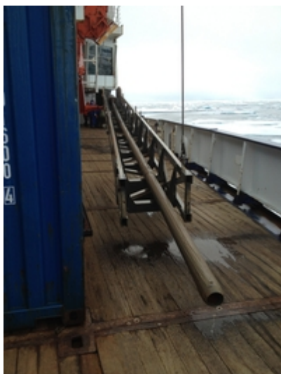
Fig. 4 Gravity core on deck. The sediment outside the core barrel indicates that the corer has been penetrated deeply. (Photo R. Stein/AWI)
