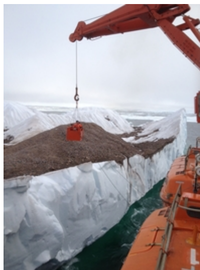
Fig. 5 Sampling the iceberg on the East Greenland Shelf, using the mummy chair. (Photo R. Stein/AWI)
