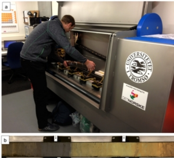
Fig. 3: (a) Matthias Forwick in his XRF-Scanner container (Photo: R. Stein/AWI). (b) Result of a XRF colour scan of a selected sediment core (Photo: M. Forwick/UoT).
