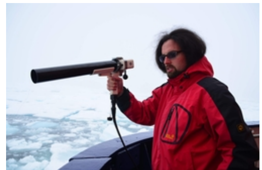
Fig. 4: Our PS87 oceanographer Albrecht Roloff (who is a geology student from Kiel University!) is working with the XCTD, measuring oceanographic data (Photo M. Winkler/AWI)
