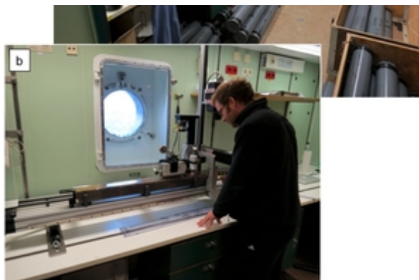
Fig. 2: Logging onboard Polarstern (Photos: R. Spielhagen/GEOMAR). (a) Laboratory 1 with MSCL-logging device and cores recovered by means of gravity corer and ready to be logged. In the back, chief-logger Frank Niessen and logging assistant Tanja Hörner. (b) Laboratory 2 with colour scanning and point-susci-device. In front of the logger Michael Schreck
