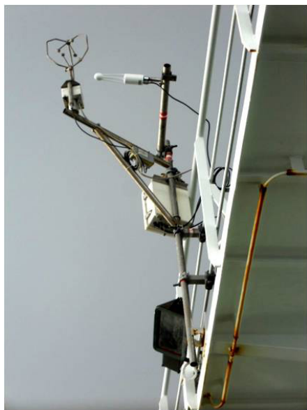
Fig. 10.1: Sonic (top left) and Licor (top, centre) mounted on the crow's nest of Polarstern.
