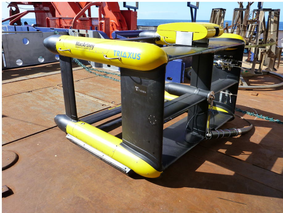
Fig. 16.1: TRIAXUS at rest on the aft deck of Polarstern after towing
