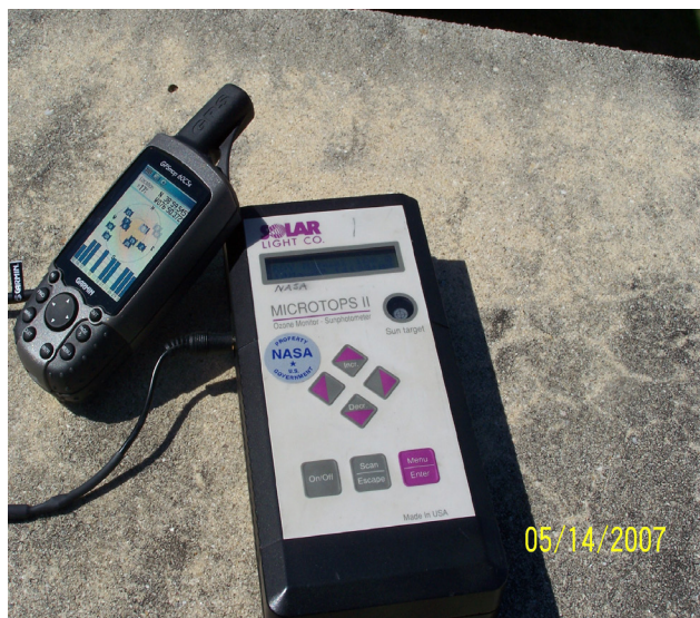
Fig. 7.1: Microtops and GPS unit provided by the Marine Aerosol Network of AERONET at NASA-GSFC.
