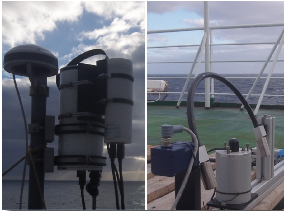
Fig. 7.2: The shadowband radiometers. The radiometer from Biospherical Instruments Inc. on the left and the self-build one at the right side
