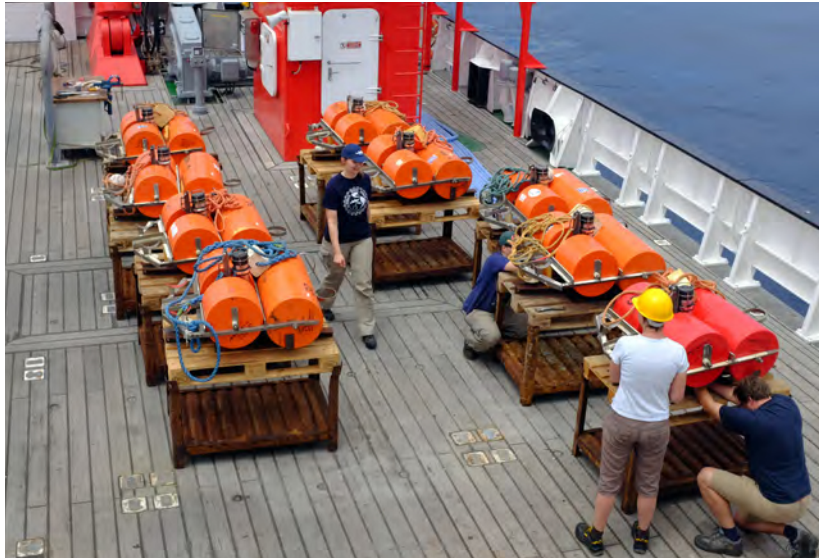
Ocean bottom seismometers are being prepared on the main deck of RV SONNE. The instruments will record the seismic activity along the Chilean plate boundary for a period of 6 months.
