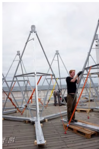
GeoSEA Tripod on the aft working deck (Height app. 4 m without transponder beacon).
