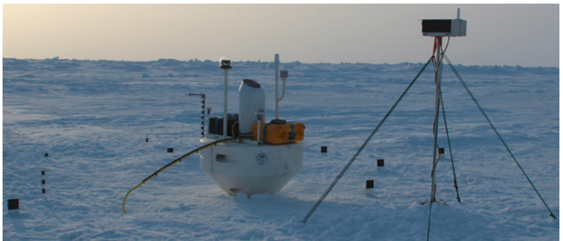
Figure 3: Complete IAOOS platform with microlidar and ODS at the North Pole in April 2014. A web camera is taking pictures 4 times a day to monitor ambient conditions.
