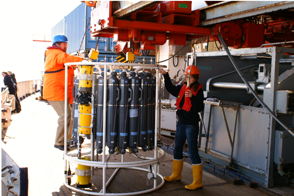
Figure 6: CTD, rosette and LADCPs on board R/V Polarstern . The yellow LADCPs, one facing upward and one facing downward, are mounted onto the rosette and measure flow speed and direction simultaneously to every CTD cast. The middle yellow pot is an additional battery pack for the LADCP system. A big steel weight is located inside the rosette (not visible here). (Photo: T. Dippe, Alfred Wegener Institute)
