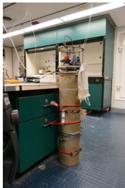
Fig. 3: The Imaging Flow Cytobot (IFCB) is able to determine the abundance and species distribution of phytoplankton
