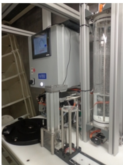
Fig. 4: Picture of the Automatic Filtration of marine Microbes (AUTOFIM) unit. 24 filters are provided in a filter magazine. Up to 5 liters of water can be sampled at a time for marine microbes. Photo: Johanna Hessel
