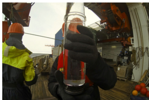
Figure 5: A sediment trap, deployed at 90 m after recovery. On the bottom of the cylinder the trapped sinking particles are visible (Photo: Christine Dybwad).
