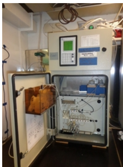
Fig. 5: Nutrient analyzer \mu MAC-C. The nutrient analyzer is connected to the Ferrybox. Phosphate, silicate and nitrate/nitrite are automatically measured by the device based on colorimetric reactions. Photo: Johanna Hessel
