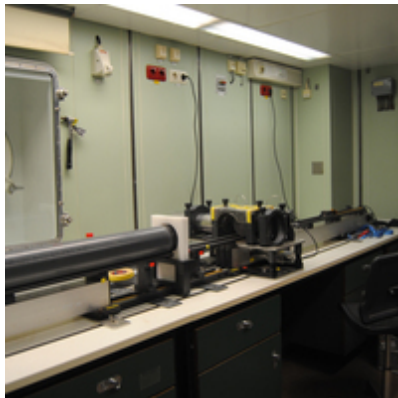
Figure 9: The Multi Sensor Core Logger measures physical properties of the sediments. (Photo: Kirstin Werner).
