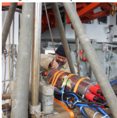
Figure 5: Winch electrician Thomas Feiertag connecting the camera system on the Multicorer to receive high resolution images from the deep sea (Photo: Jens Matthieß).
