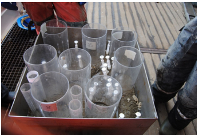
Figure 7: Sediment sampling of the box core using different tubes and syringes (Photo: Kirstin Werner).
