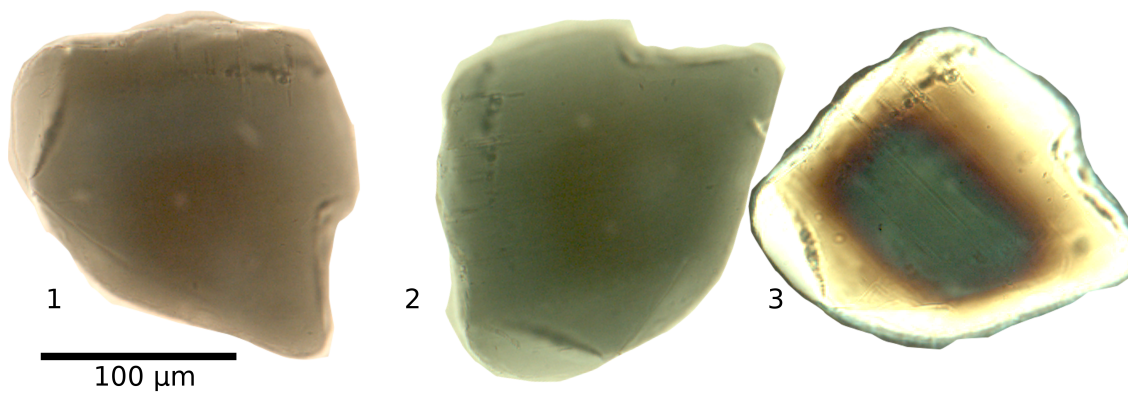
Figure A.8: Microscopy pictures of hornblende: (1) single-polarized light, (2) single-polarized light, 90° rotation, (3) crossed polarization filter
