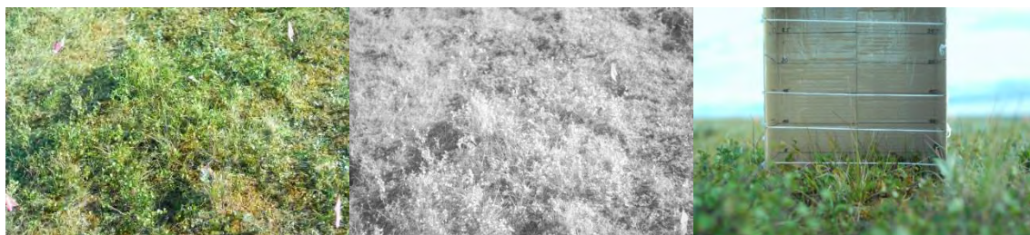
Figure C.7-4: Overview images of the VDG1 vegetation. Left: Photo in the visible wavelength range. Middle: Photo in the NIR wavelength range. Right: Vegetation height measurement with help of the card box approach. Source: [Heim et al. , 2012]
