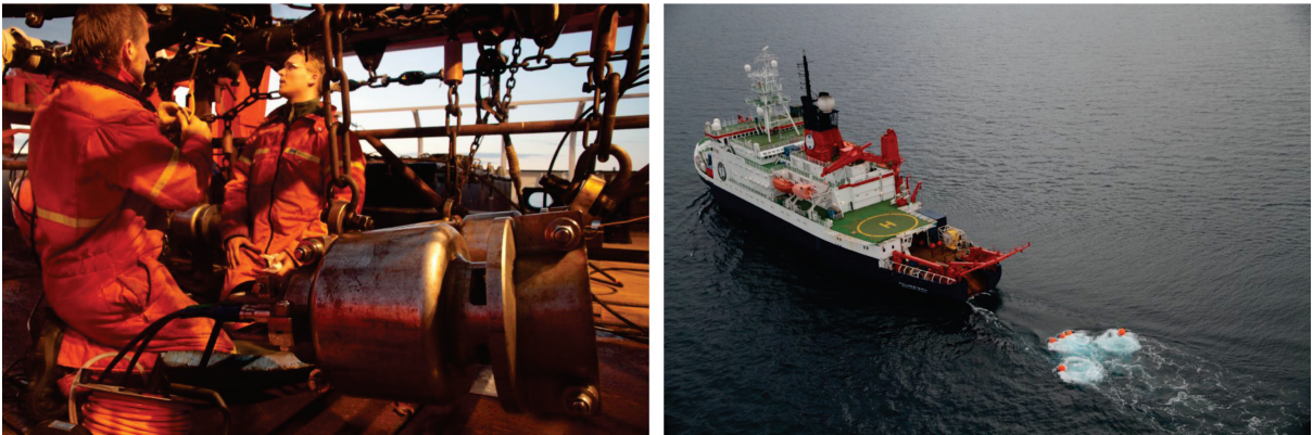
Figure 3: Airgun array used during expedition ANT-XXIII/4 in 2006.
