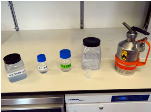
Common fixatives for zoological specimens include (from left to right) 4% solution of formaldehyde (or formalin), mixture of acetone and methanol (ACME), 4% solution of paraformaldehyde (PFA), RNALater, and 100% ethanol (EtOH). (Alexander Ziegler)
