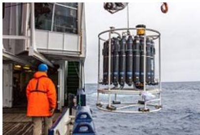
Fig. 1: The last CTD with acoustic current meter goes into the water. (Photo: Thomas Ronge, AWI)
