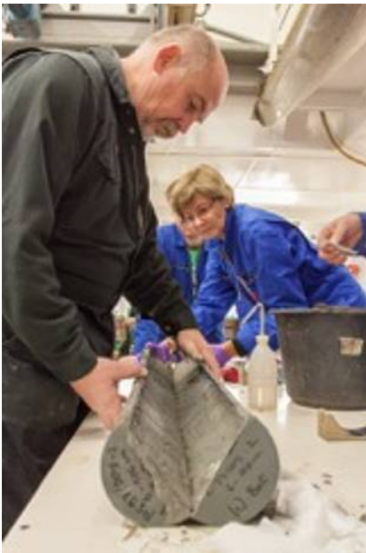
Fig. 2: Work in the geolab has begun. Dirk Nürnberg (GEOMAR) and Carina Lange (University of Concepción) splitting a core section. (Photo: Thomas Ronge, AWI)
