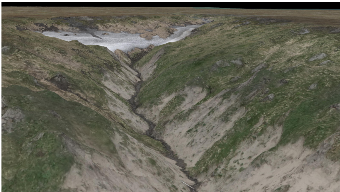
Figure 2.12.-4: DEM sample of Kurunknakh island sideview with surface texture; resolution of a base orthophoto image ~7 cm/pixel
