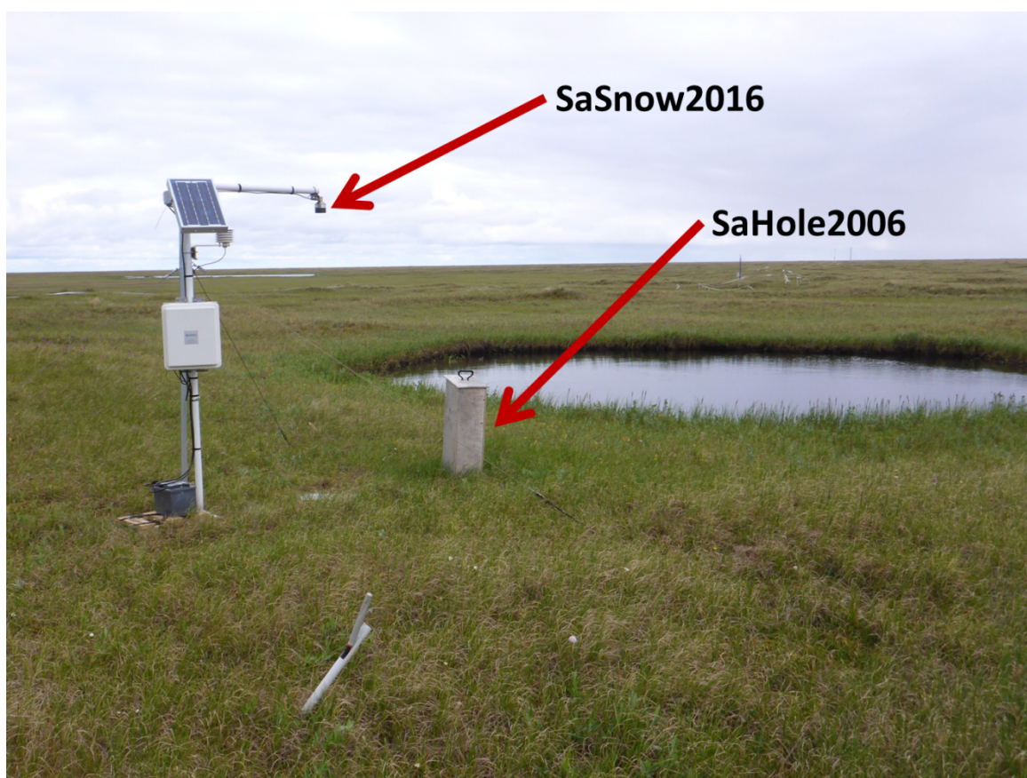
Figure 2.3.-1: Setup of the new snow depth measurement station (SaSnow2016) next to the 27m temperature borehole 2006 (SaHole2006)
