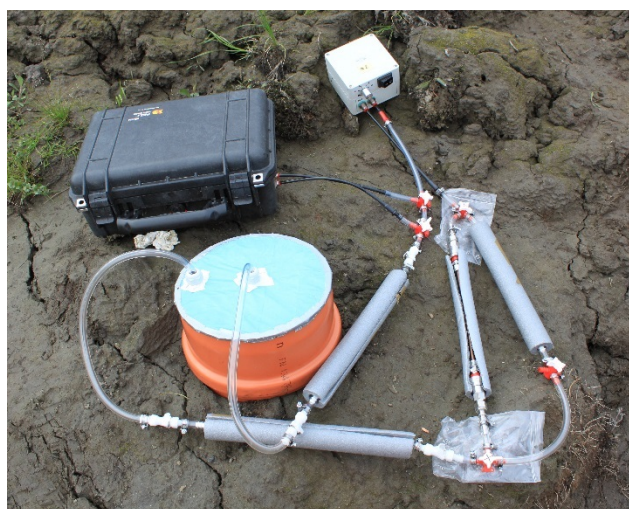
Figure 2.10.-1: Picture of our closed loop respiration chamber to which an infrared gas analyser, water traps, and the molecular sieve for CO 2 concentration are connected.
