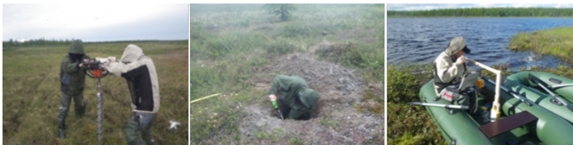
Figure 4.2.-4: (Left) Field images from permafrost coring, (middle) digging pits in the active layer, (right) ground penetrating radar profiling in the lake
