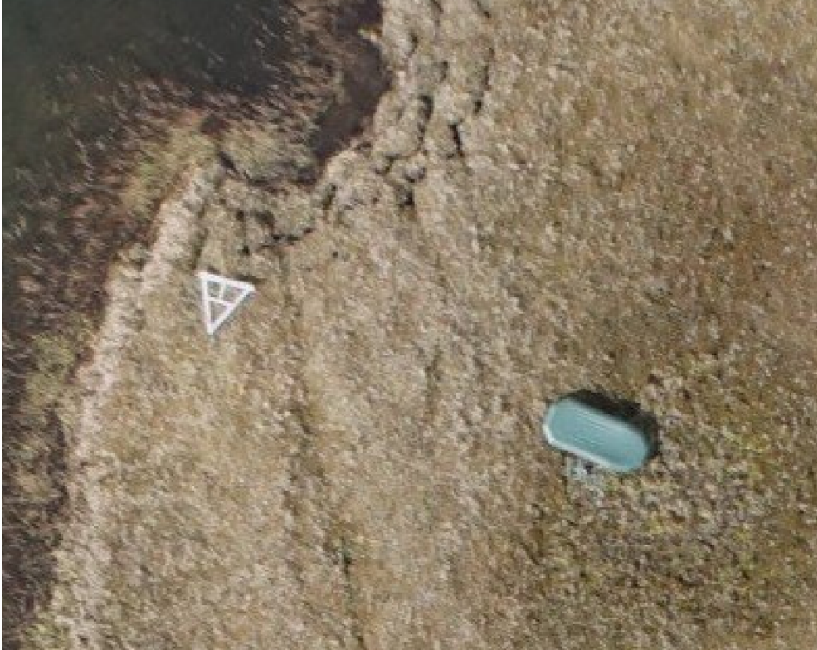
Figure 2.12.-2: Example of an orthophoto image (rubber boat can be clearly seen near the lake); resolution 5 cm/pixel
