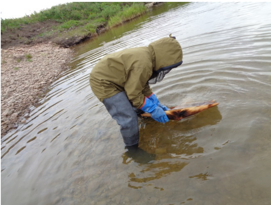
Figure 4.3.-2: Sieving and enriching the heavy mineral fraction from river sediment
