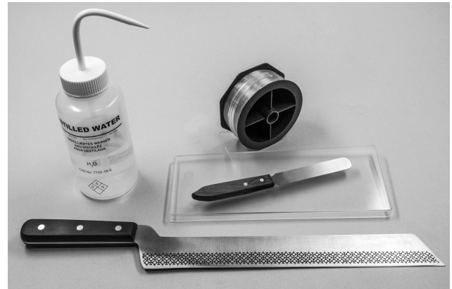
Figure 4. Equipment used for the preparation of sediment slabs for X-ray imaging comprise fishing line, distilled water, cheese knife, spatula and special Plexiglas lids for support of the sediment slab. Lids used for preparation measure 25 cm × 10 cm × 1 cm (Bensberger Kunststoffwerk Lappe GmbH). Lay-flat tubing and sealing device (not shown) are used to protect the sample from drying.
