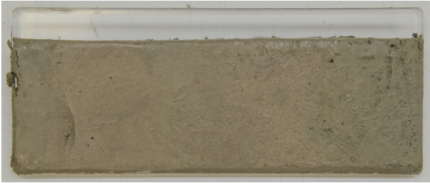
Figure 2. Sediment slab (25 cm × 10 cm) stabilized in Plexiglas lid ready for X-raying. Top of core is to the left.
