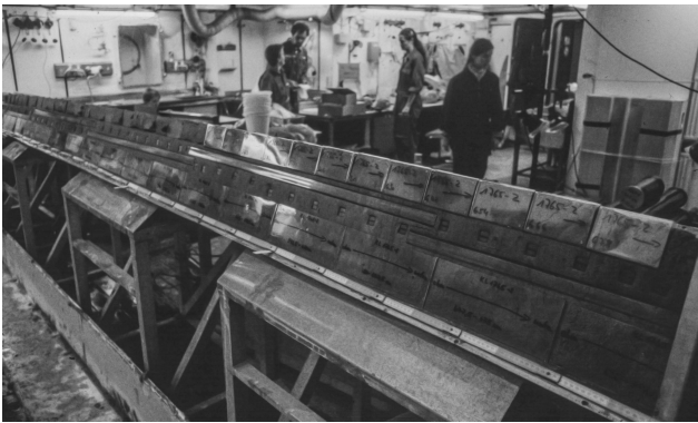
Figure 3. Sediment core taken with a kasten corer (30 cm × 30 cm) prepared with Plexiglas lids to remove the samples for X-raying.
